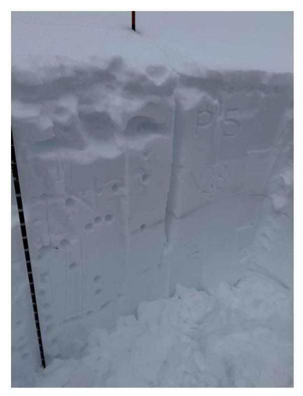
We dug a snowpit near the lower flank of the avalanche path and noted that these weak layers had gained strength over time. We did get propagation on a stout melt-freeze crust near the surface (ECTP5) but did not get propagation lower down on faceted grains. Photo: GNFAC
