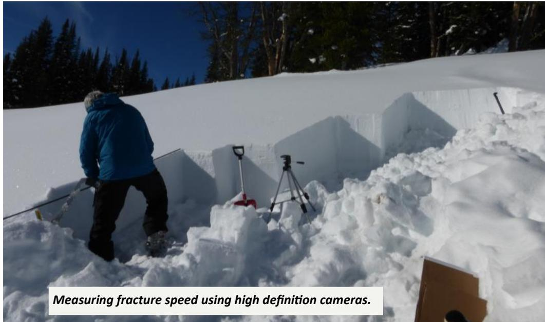
*Measuring fracture speed using high definition cameras.*
